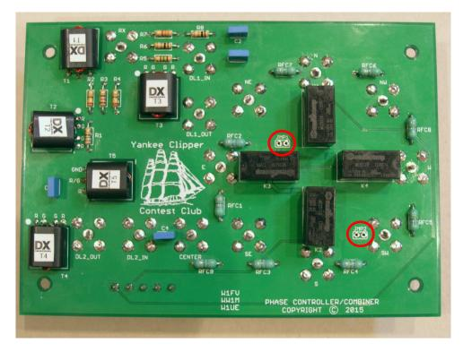
Figure 16.Component side of combiner PCB (jumper locations circled in red—see text)
