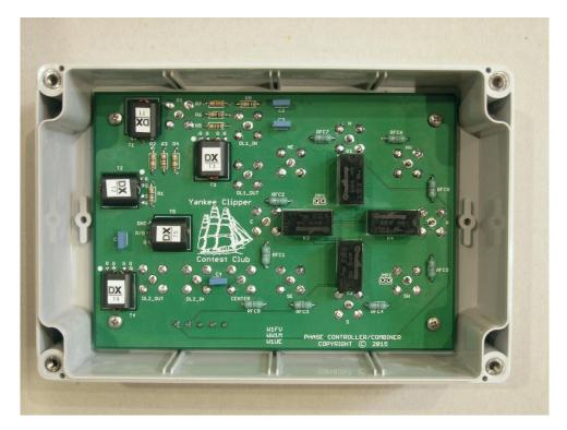
Figure 20. Inside view of PCB mounted in enclosure
