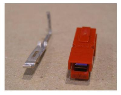
Figure 22. DC power connector body and pin
