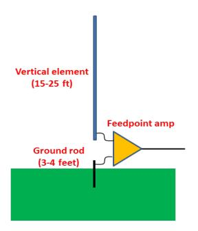
Figure 6. An "active" receiving antenna
