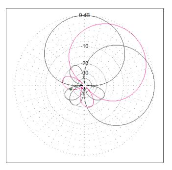
Figure 5. Pattern overlap of 9-element array
