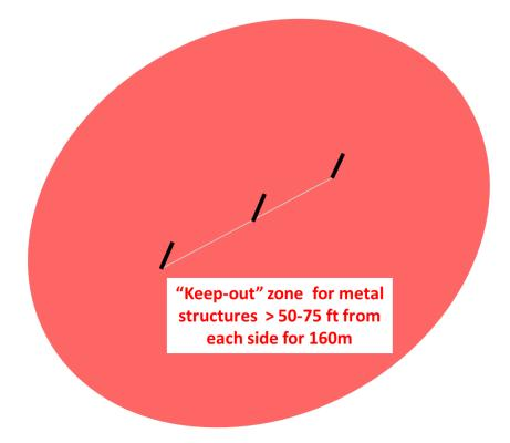
Figure 8. "Keep out" zone for 3-element inline system
