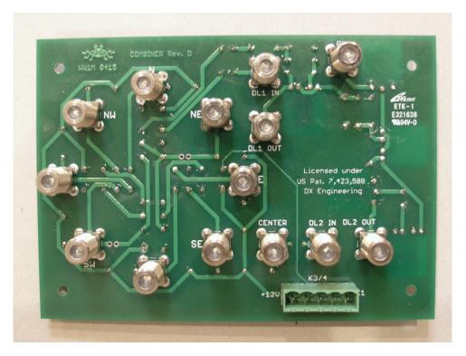
Figure 17. Bottom side of combiner PCB
