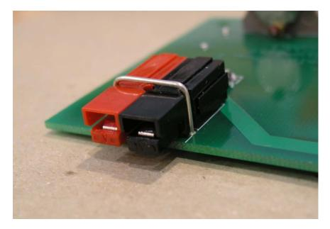
Figure 25. Wire staple holding power connector to PCB
