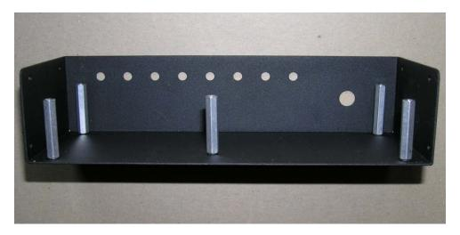
Figure 30. Mounting of aluminum standoffs
