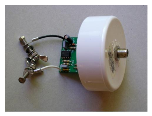
Figure 12. Preparation of end cap for preamplifier enclosure
