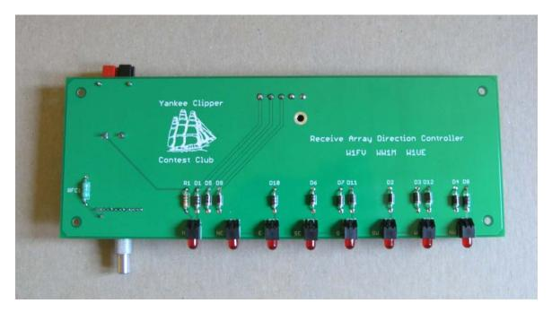
Figure 26. Top side of direction controller PCB
