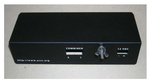
Figure 32. Ground terminal screw on rear panel
