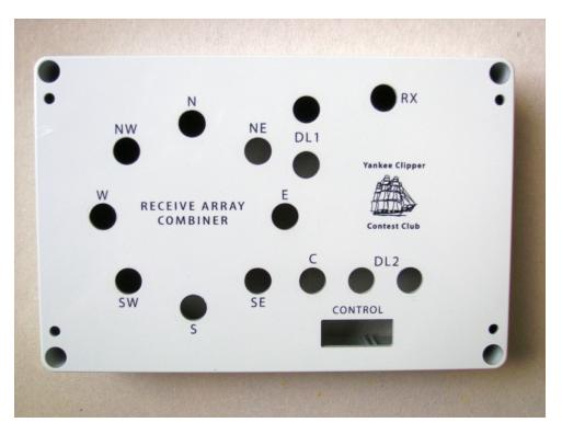
Figure 18. Bottom view of pre-drilled combiner enclosure
