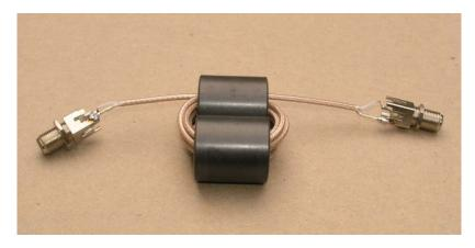
Figure 36. Feedline choke winding
