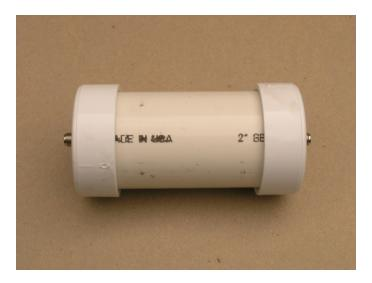
Figure 37. Completed feedline choke
