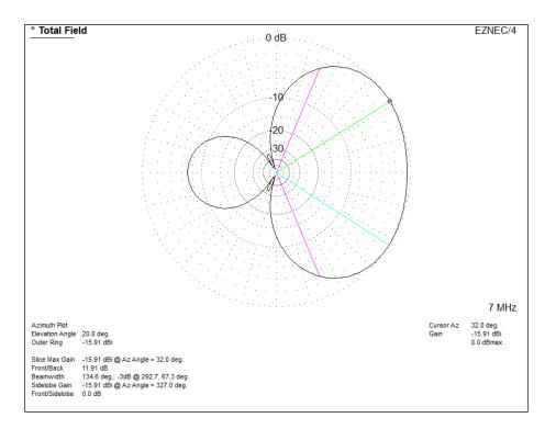
RDF @ 20 degree elevation = 9.1 dB
