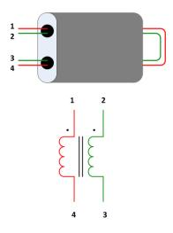
Figure 15. Bifilar winding technique
