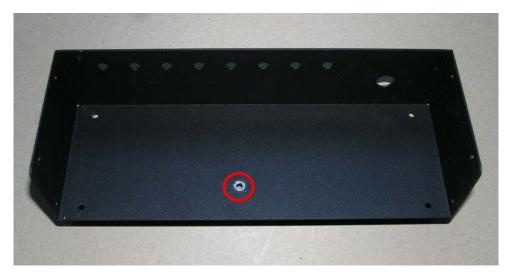
Figure 29. Scrape away paint around hole encircled in red
