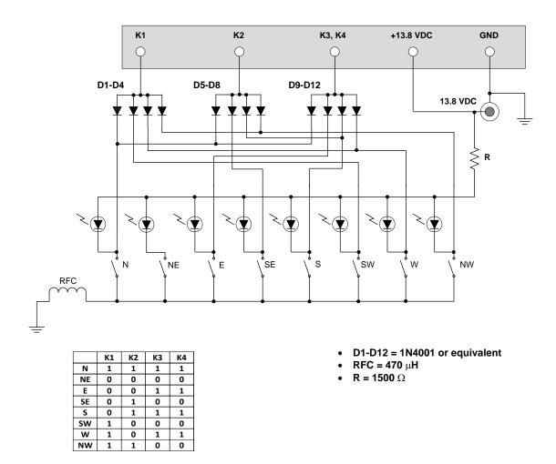
Figure 43. Direction switch controller
