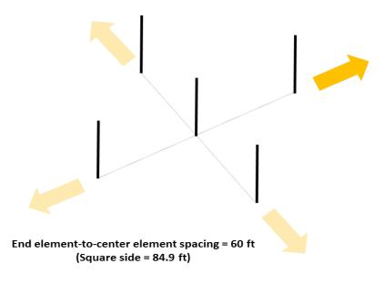
Figure 2. 5-element square configuration
