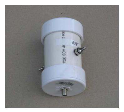
Figure 14. Completed feedpoint preamplifier
