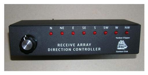
Figure 33. Front side of finished direction controller unit
