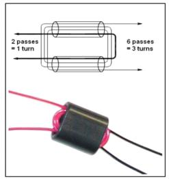
Figure 10. Transformer winding technique
