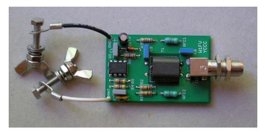
Figure 11. Feedpoint preamplifier PCB
