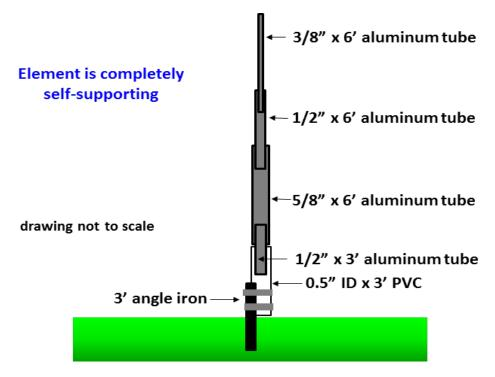
Figure 9. Construction of an aluminum tubing vertical
