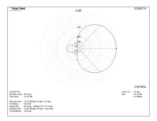
RDF @ 20 degree elevation = 11.3 dB
