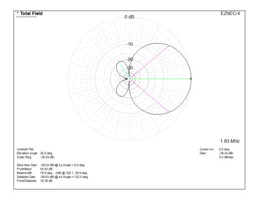
RDF @ 20 degree elevation = 12.1 degrees
