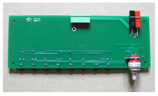
Figure 27. Bottom side of direction controller PCB
