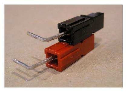
Figure 24. DC power connector bodies being joined together
