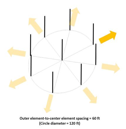
Figure 3. 9-element circular configuration
