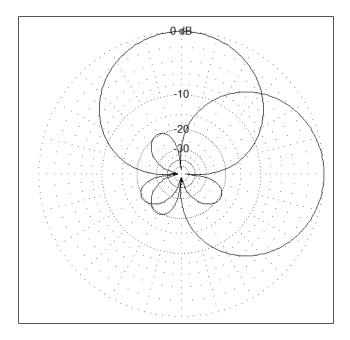
Figure 4. Pattern overlap of 5-element array
